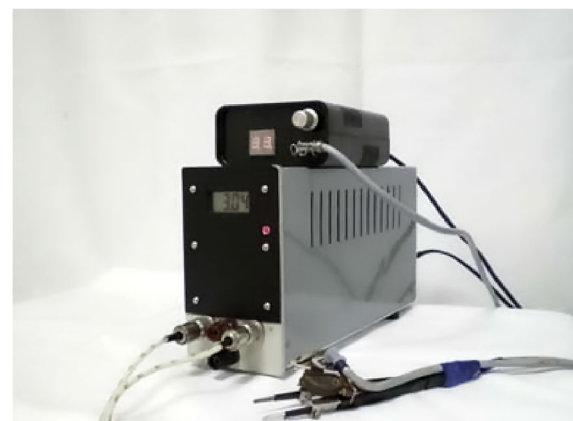
Fig. 2 Russian-made experimental bioimpedance meter for surgery and military surgery [39, 40]
